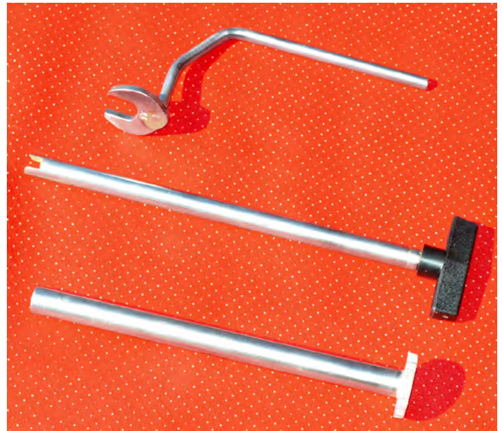
Special set of tools for Guilietta shock absorbers on Guilietta red vinyl seat fabric
