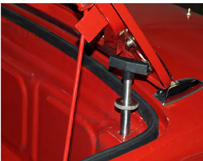
Inserting the two parts of the combination rear shock absorber installation and adjustment tool
