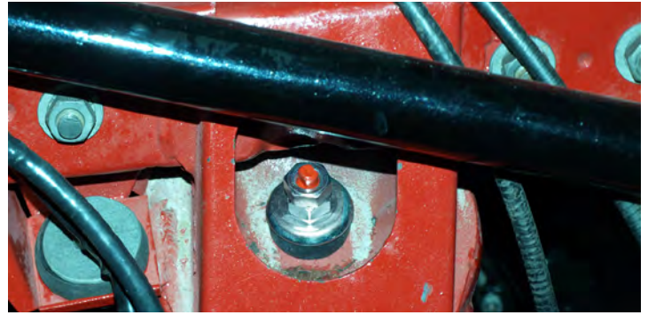
Steering column rod makes access to the recessed front driver-side shock absorber mount more difficult
