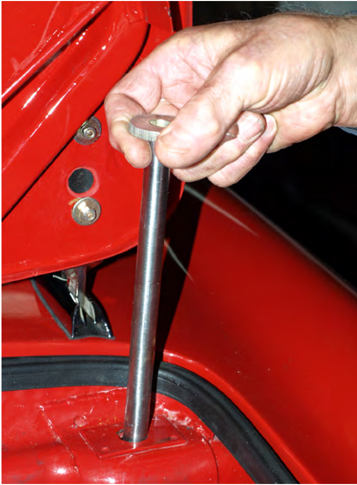
Steering column rod makes access to the recessed front driver-side shock absorber mount more difficult
